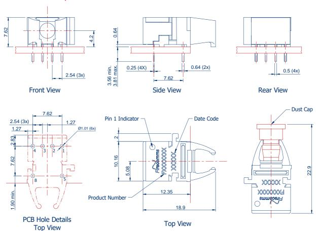
FIGURE 6 Mechanical dimensions of the horizontal connectors and PCB footprint, which is a top view General dimensional tolerance is  $\pm\,0.2~\text{mm}$
