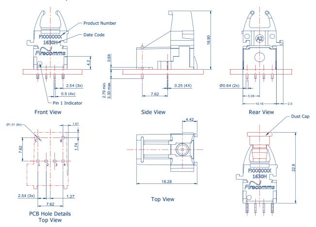
FIGURE 8 Mechanical dimensions of the vertical transmitter connectors and PCB footprint, which is a top view General dimensional tolerance is  $\pm\,0.2$  mm
