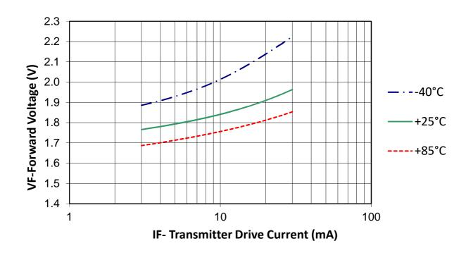
FIGURE 4 Typical forward voltage (VF) vs. drive current (IF,DC).
